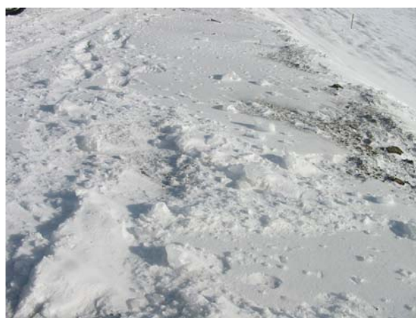
Fig. 35: Impact in snow from falling ice
