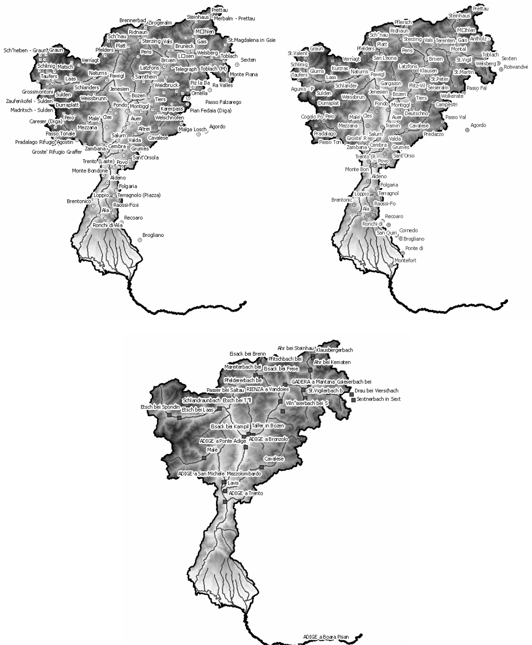
Figure 16. Input data for TOPKAPI model. Upper left: the 129 rain gauges in the Adige Basin. Upper right: the 171 thermometers on Adige Basin. Bottom: hydrometric stations.
